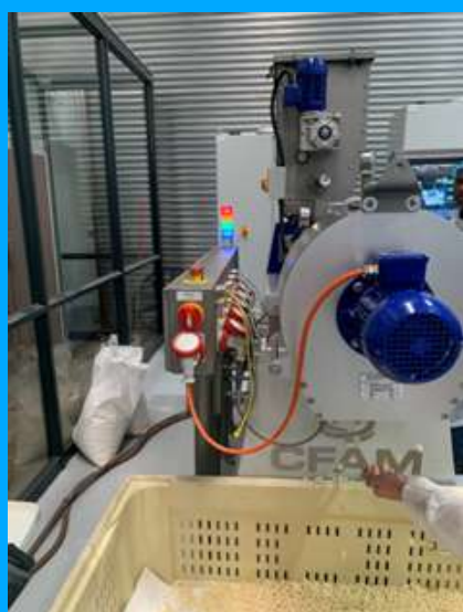
Trial products produced on a new twin screw extruder system by UNAM
