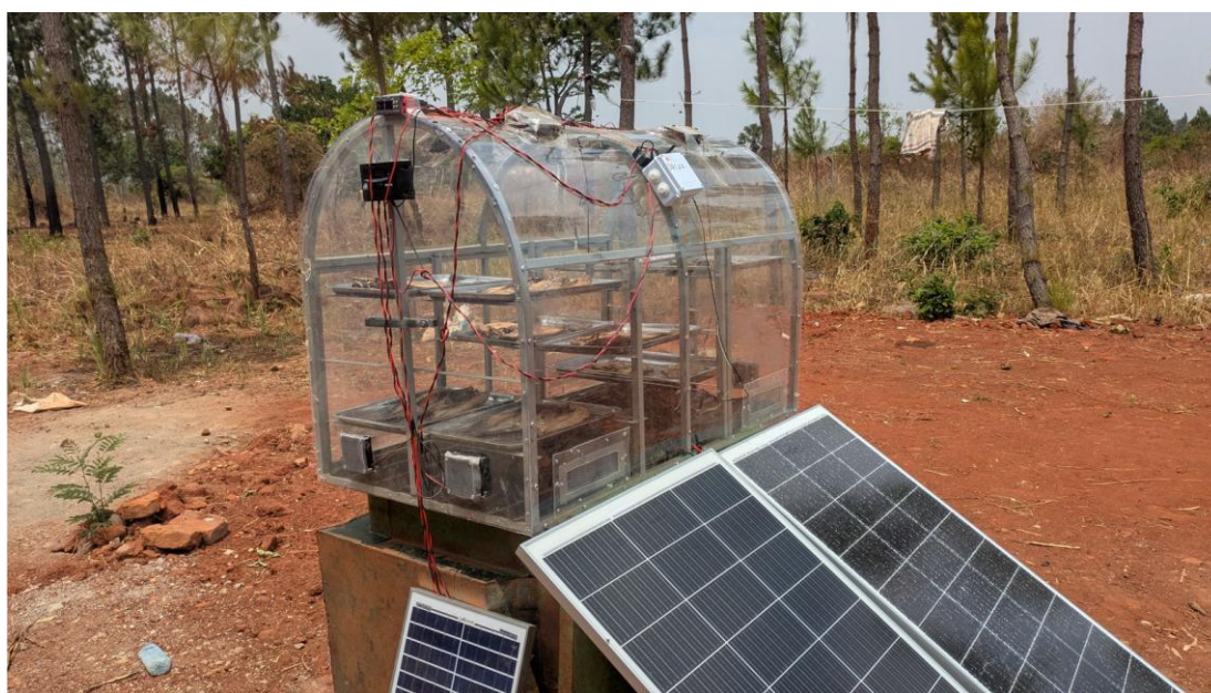
Figure 3. Photos of the Sparky Smart Solar Dryer with PV panels and fans for ventilation [LO2025].
